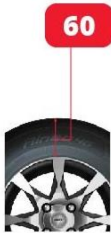
Profile = 60% described aspect ratio – the ratio of the height to width in percentage
