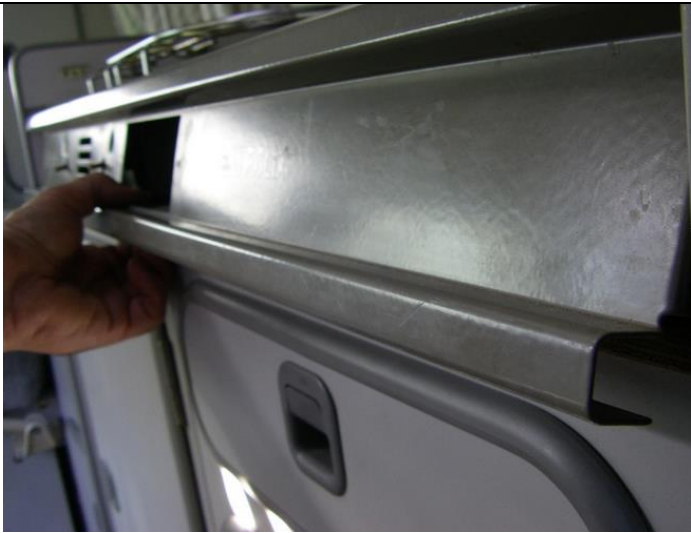
Carefully pull the bottom of the faceplate away from the cabinet
