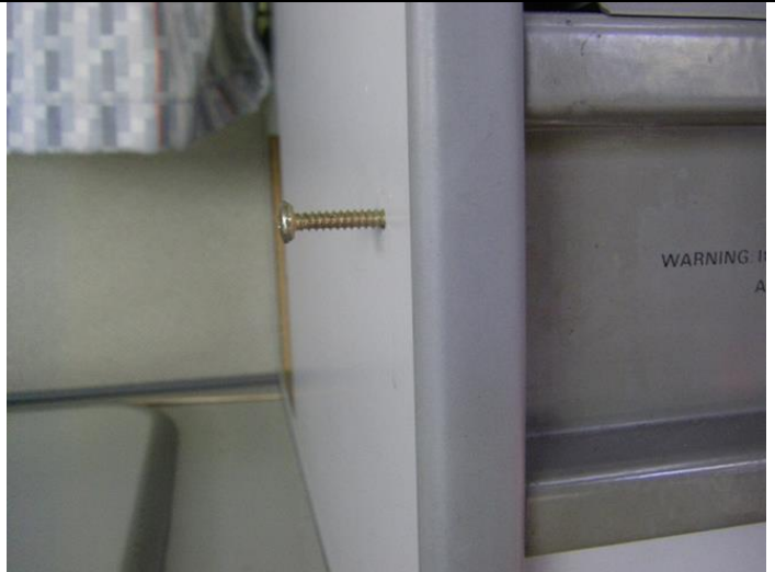
Remove 3 Philips screws beneath panel
