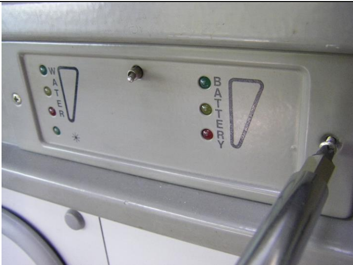
Remove Philips screws from LED panel
