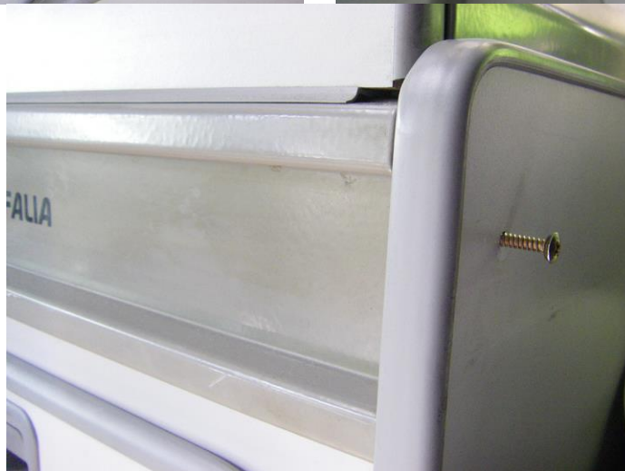
Remove screw caps from front and rear kitchen panels and remove the two Philips screws
