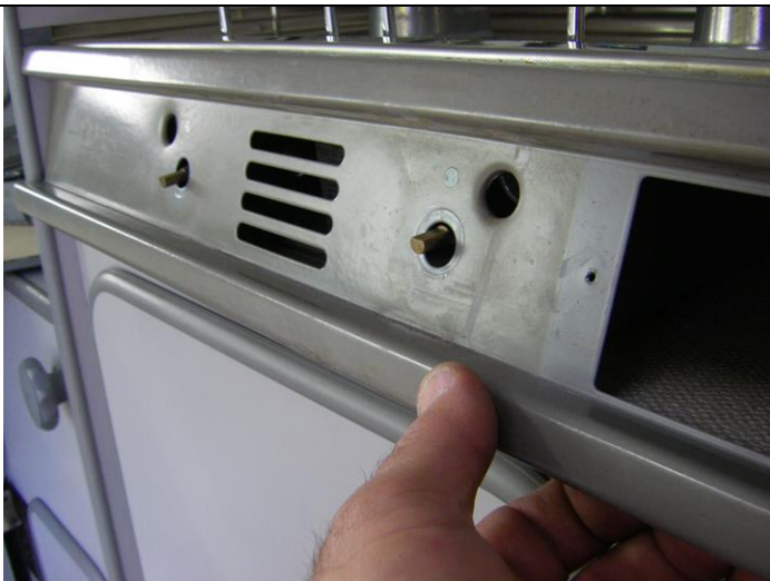
Keep an eye on the valve stems – faceplate may catch on the threaded part of the valve stems
