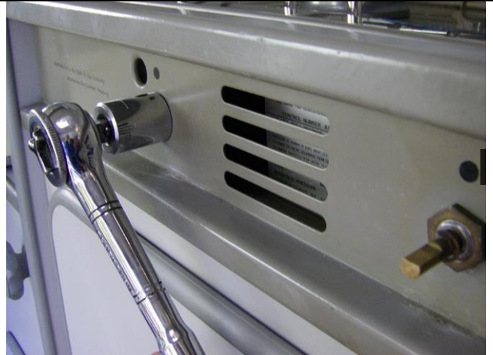
Remove valve retaining nuts (17mm)
