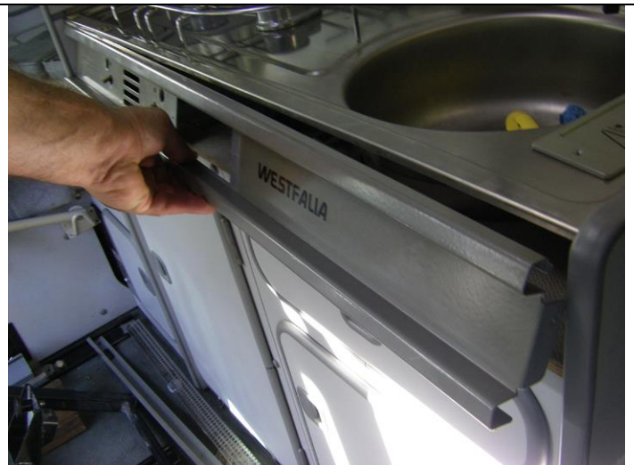
Carefully pull the stove face down and away from the cabinet
