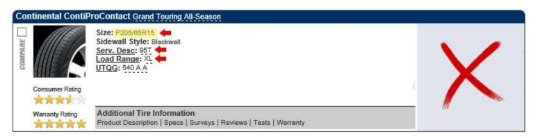
The tire's load index is 95, which means 1521 lbs. It is a P-metric tire, which means reducing that 1521 lbs. by 9%, which equals 1384 lbs. – too low for van use. Bottom line: Be vigilant when shopping for P-metric tires for your van.
