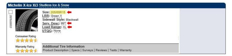
To recap: Any tire that is not designated as LT (light truck), or does not have a C or higher load range, must undergo the 9% reduction in max load weight. However, it is unclear at this point whether a P- or Euro-metric SUV-branded tire (such as the Yokohama Geolandars) with an SL or XL rating must also undergo the 9% reduction.
