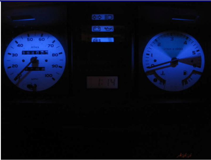
Member: ahollon Speedo, tach, warning lights, clock: Blue LED White gauge faces installed.
