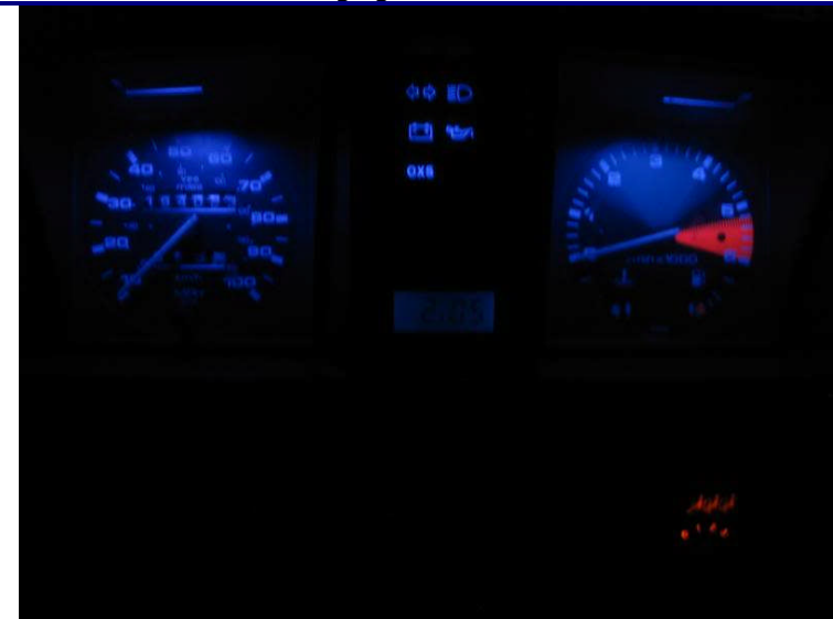
Member: ahollon Speedo, tach, warning lights, clock: Blue LED Switch: Red LED
