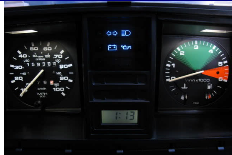
Member: kamzcab86 Speedo, tach, clock: White LED Warning lights: HP Blue LED
