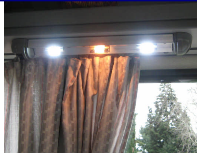
Member: ANGOVAY Westy kitchen light: Center is original incandescent; right & left are new LEDs
