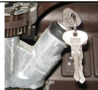
Insert key into ignition switch – leave in *off* position.
