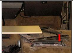
Disconnect the main battery using 10mm wrench. Use a towel, or something similar, to keep the battery ground terminal from touching the connector.
