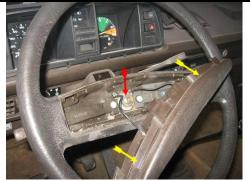
Carefully pry out center horn button pad (3 tabs across the top and bottom). Disconnect horn wires from button pad.
