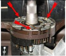
Remove the 3 slotted screws from the wiper/turn assembly and remove them both from the steering column.
