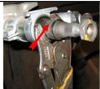
Using Vice Grips and a twisting-pulling motion, pull the spacer sleeve off the column shaft (this spacer sleeve is **plastic!** – do not use a really tight grip, or you'll ruin the spacer); or, use a proper puller tool.
