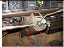
Smack the back of the steering wheel with your hand, or deadblow hammer. Once it breaks loose, remove 24mm nut and steering wheel. Using a small flat screwdriver, gently pry the upper column cover's retaining tab up and over the key lock cylinder and remove the cover (slide it off the wiper stalk).
