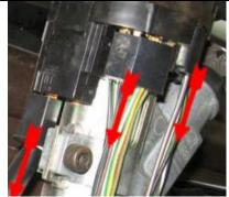
Remove electrical connections from all switches.
