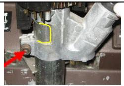
Using a Sharpie pen, mark on the steering colum shaft where the lock cylinder housing sits (yellow line; do top and/or bottom, your choice). Remove the 6mm Allen bolt and pull lock cylinder assembly off the shaft (you may need to pry the bolt-side mounting tabs apart just a bit).
