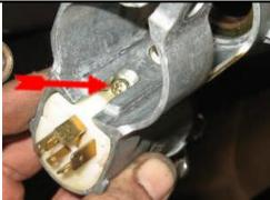
Remove the Philips screw from the ignition switch. Install the new switch and screw.
