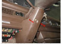
Remove the 2 Philips screws holding the steering column covers together and remove lower cover.
