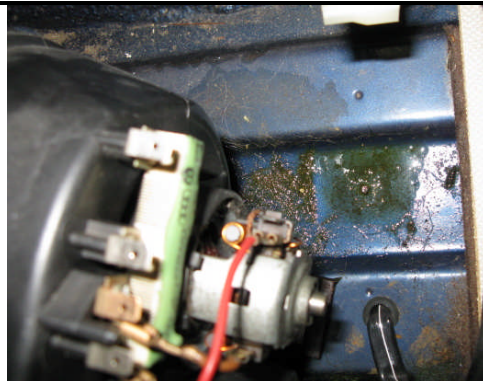
Keep your rags handy and remove the rear heater assembly, keeping the heater core's hose flanges up. Drain the remaining fluid into an appropriate container and dispose of properly. What you should now have under the rear seat is shown above (with more or less of a mess).
