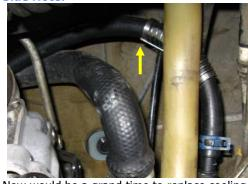
Now would be a grand time to replace cooling components: old hoses, temp senders, etc. I took the opportunity to replace the temp II sender (leaking & original!) and the crossover hose, which was completely collapsed at the bend (installed a spring support on new hose).
