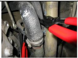
Pick one of the two heater hoses (location: above plastic pipes, right side of transmission) and remove (by sliding them back several inches) the two hose clamps on each side of its T-fitting. Pinch off each hose on both sides of said T-fitting.
