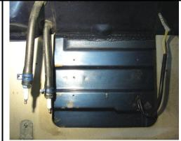
Clean up the mess left by the leaking heater. If the leak was really bad, and depending on your van, you may need to remove the wood/carpet floor for complete cleanup.
