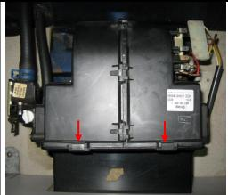
Pry off the two metal clips (red arrows) holding the blower assembly to the duct using a small flat screwdriver. Remove the duct.
