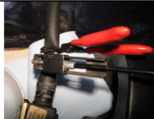
Close the valve, if not already shut (move lever towards rear of van). Put your rags into position and pinch the top hose shut, remove the top hose clamp, remove the top hose. When the coolant has drained, insert spark plug into hose, replace hose clamp, and remove pinch tool. Repeat hose removal process with bottom hose.
