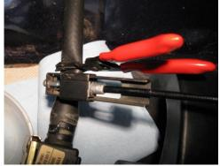
Close the valve, if not already shut (move lever towards rear of van). Put your rags into position and pinch the top hose shut, remove the top hose clamp, remove the top hose. When the coolant has drained, insert spark plug into hose, replace hose clamp, and remove pinch tool. Repeat hose removal process with bottom hose.
