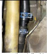
Carefully remove the main (front) heater hoses from the T-fitting (warning: coolant will spill out!) and insert your new straight fitting. Remove the hose pinchers and replace the hose clamps. Pull the rear heater hose out (remove hose clamp and plug first, if still in place). Drain remaining coolant. Repeat process with second hose.
