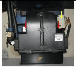
Remove the white electrical connector (yellow arrow). Remove the two blower assembly screws from the floor (red arrows). Note: There is a block of wood under each bracket that may be soaked in coolant.
